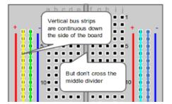
The two columns along the side are for powering the board. You will notice a (+) on one side and a (-) on the other. When connecting a battery pack, the red wire goes to (+) and the black wire goes to (-).
